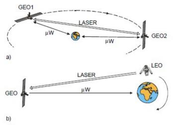
Fig. 5 Two geostationary satellites (GEO1, GEO2) are connected by a laser duplex link (a). A low-earth orbiting satellite (LEO) transmits data via a laser link to a GEO acting as data relay (b). In both cases the downlink is via microwaves ( $\mu$ W).<sup>5</sup>
